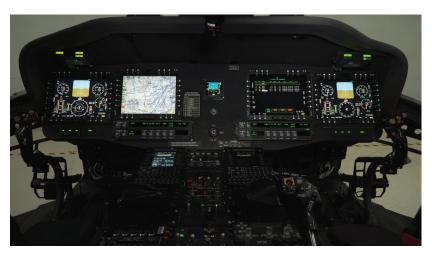
The UH-60V cockpit features Northrop Grumman's software-defined mission equipment package with a digital, open architecture integrated glass cockpit. *Photo credit: Northrop Grumman*
