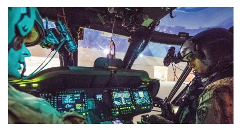
Northrop Grumman provides the Integrated Avionics Suite for the UH-60V, a modernized technology supporting rapid and timely capability enhancements and replacing the analog gauges in UH-60L helicopters. *Photo credit: U.S. Army*
